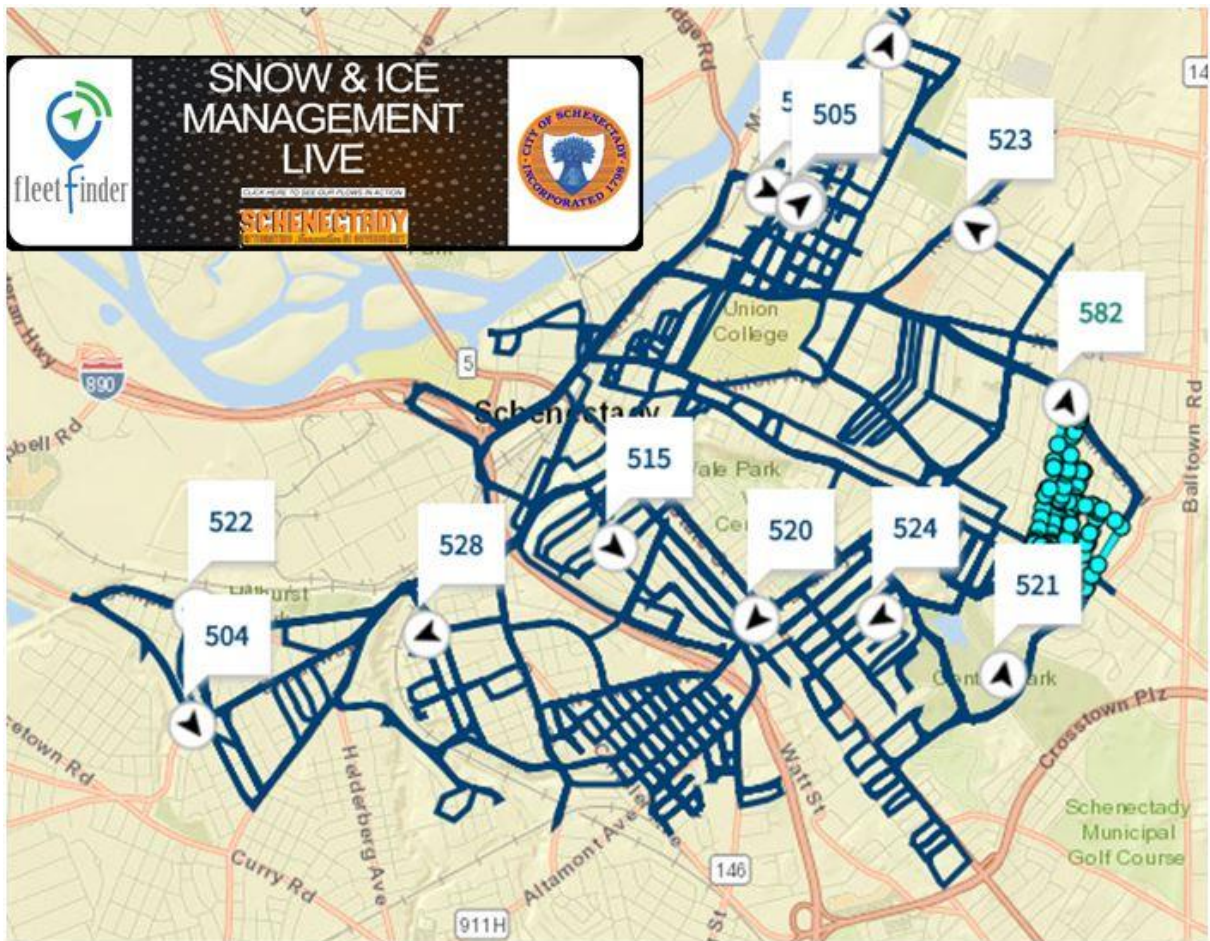
Screenshot of FleetFinder taken on November 16, 2018. The blue routes indicate where snowplows have been in the last four hours.
